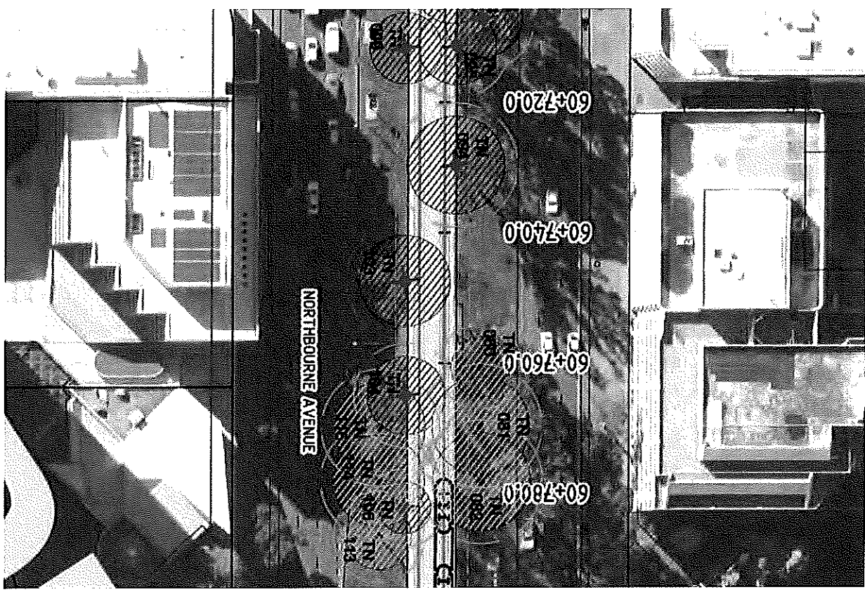
Figure 5: Showing tracks (grey), construction zone offset (orange line) and TPZs (blue circles)
