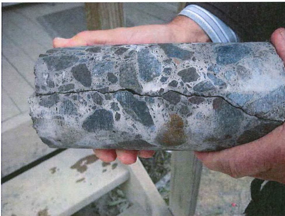
Photograph 5.4 The full core into the lower crack. Note the crack initiating off the lift joint.
