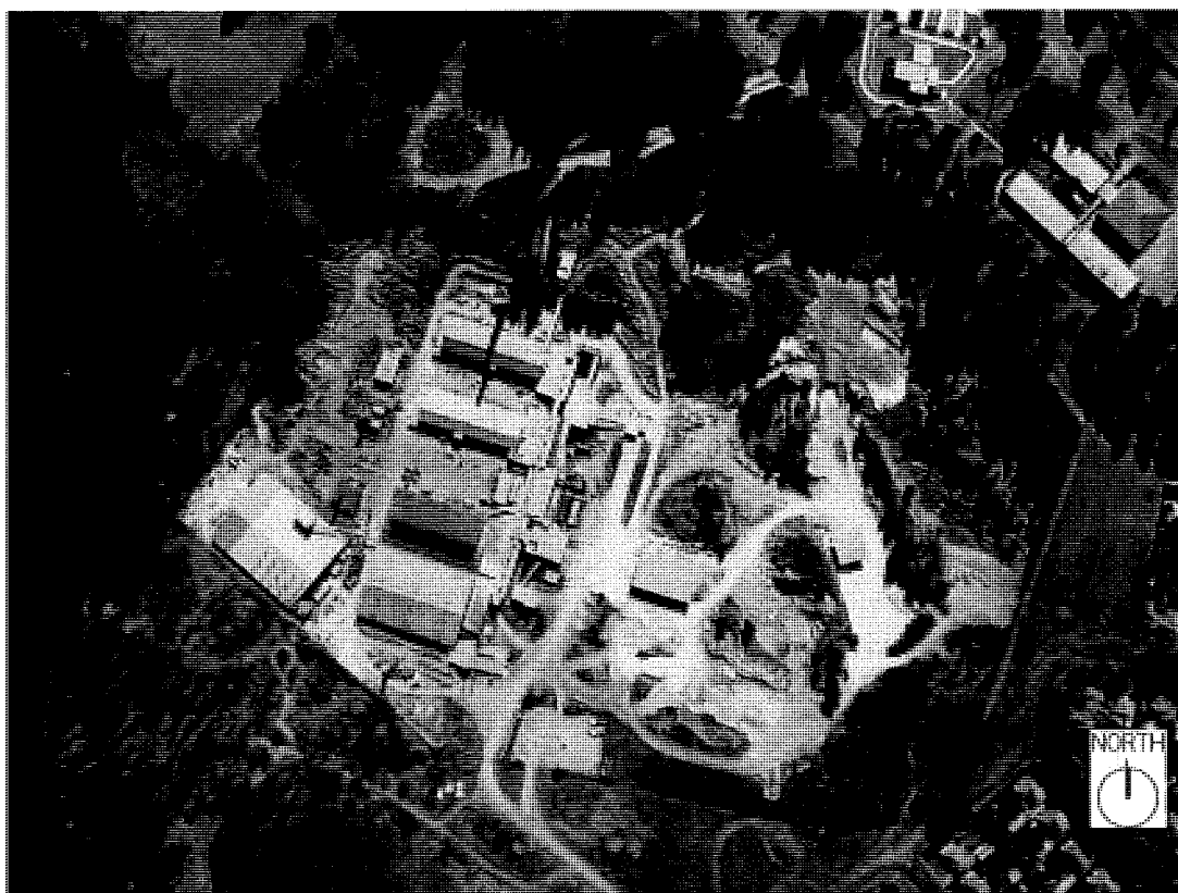
Figure 7 Aerial view, c.1976, at the time of the closure of the Canberra works. At this date, the raw materials had for many years been brought onto the site but the process continued to occur moving from east to west across the site. The 'spine' of process buildings (grinding, crushing, pressing) was located east of the kilns (between the kilns and the quarry). Source: ACT Heritage Library
