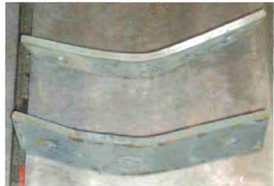
End Plate after test
