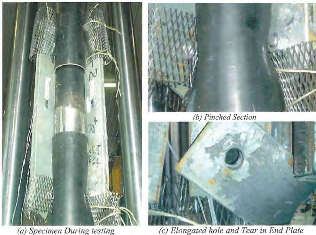
Figure 45 – Failure of Specimen 8
