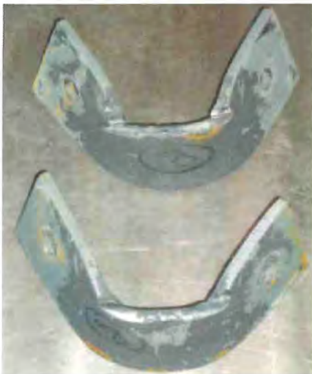
End plates after test
