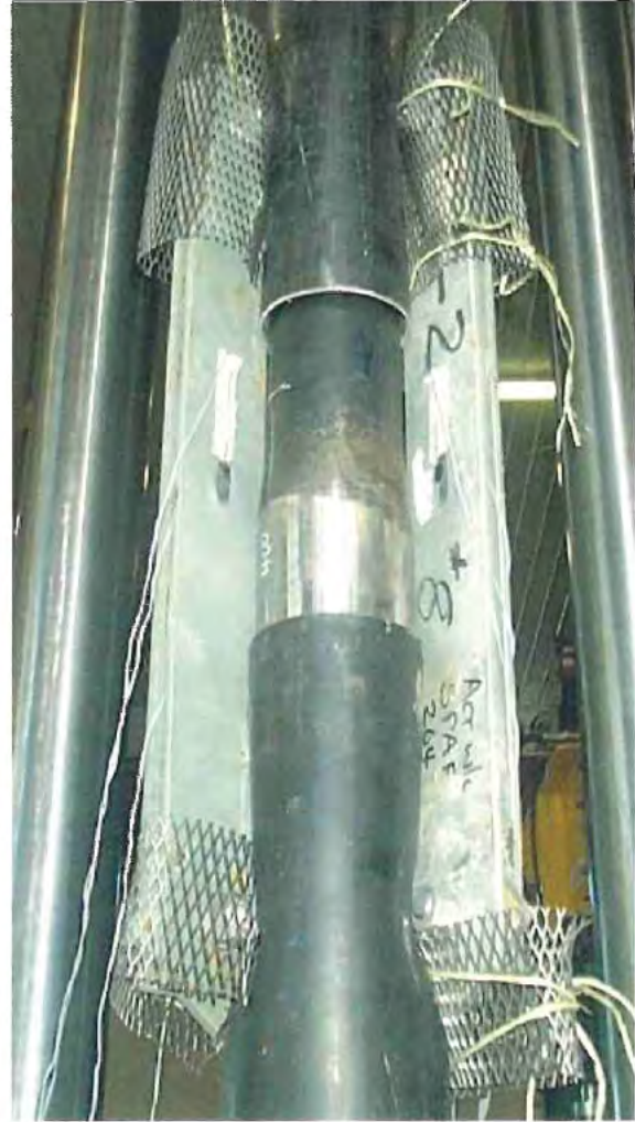
Deformations at peak load
