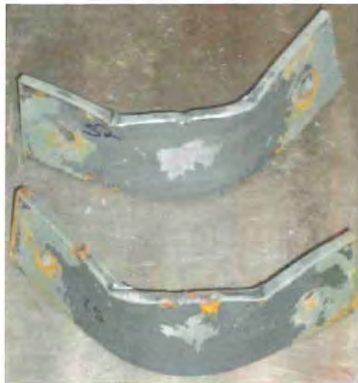
End plates after testing.
