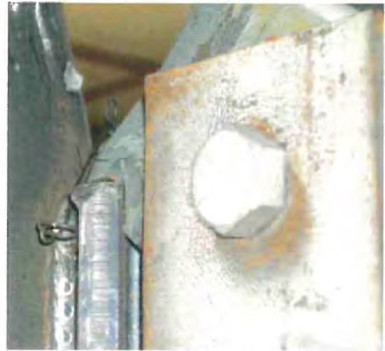
Endplate at peak load
