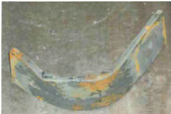
End plates after test
