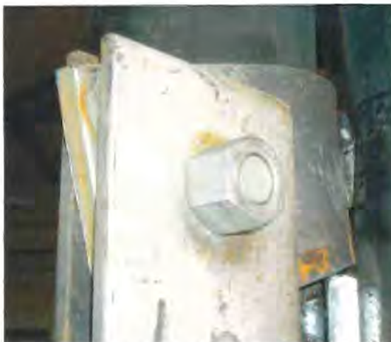
(b) Typical Deflections of the End Plates
