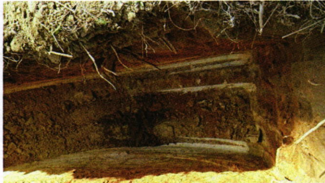
Photograph 9: Orange brown and yellow brown clays typical of the residual soil overlying dacite. TP8.
