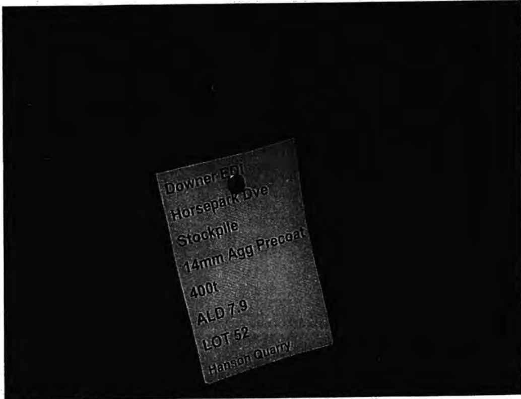
Image 03: Pre-coated aggregate for the 14/7mm seal delivered to site by Hanson
