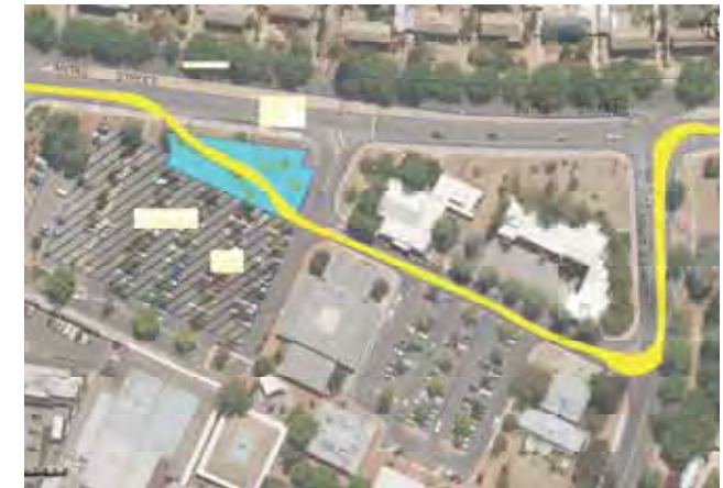
Figure 11: Services vehicle 'swept' path
