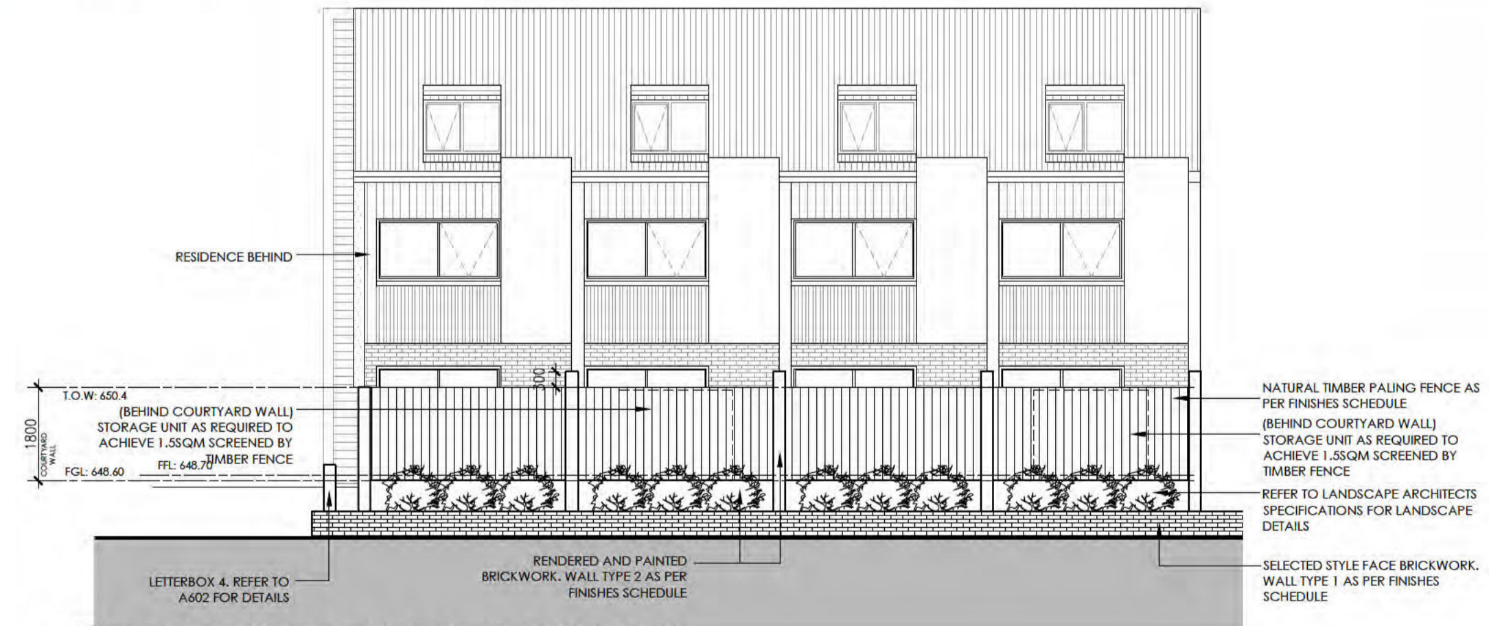
COURTYARD WALL ELEVATION 1:100 @ A1
