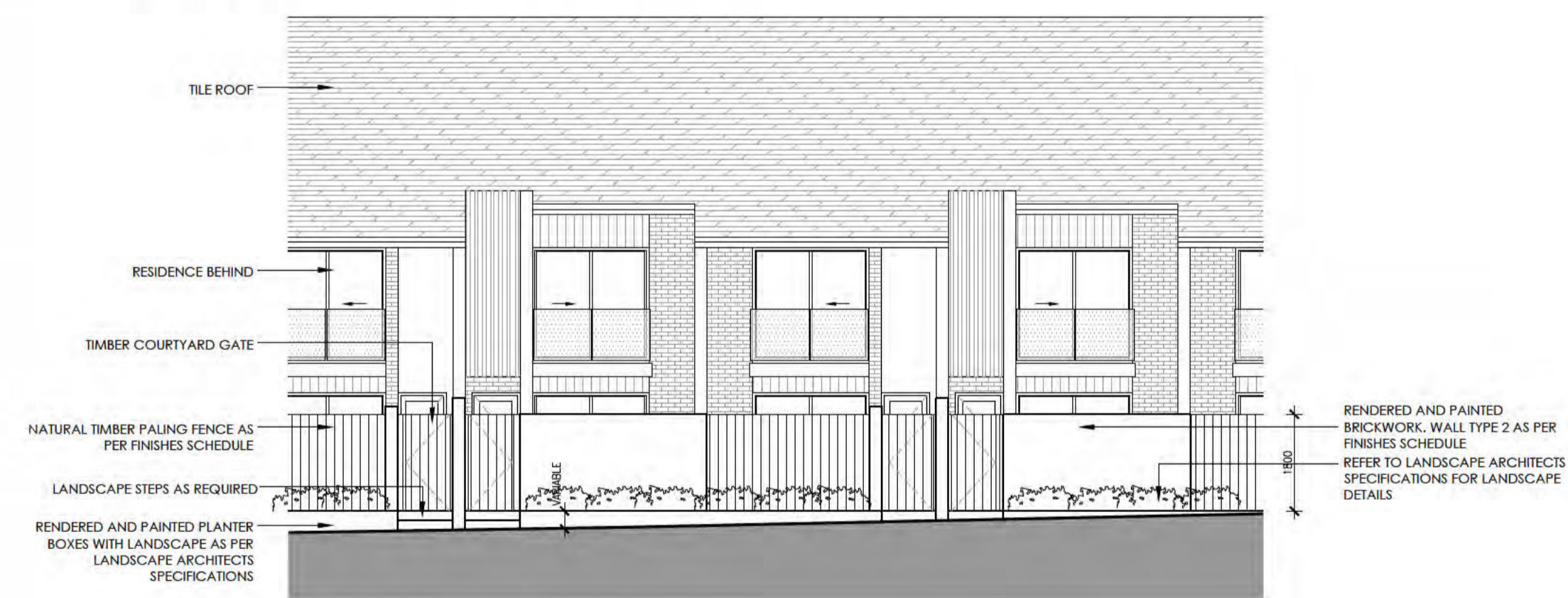
COURTYARD WALL ELEVATION 1:100 @ A1
