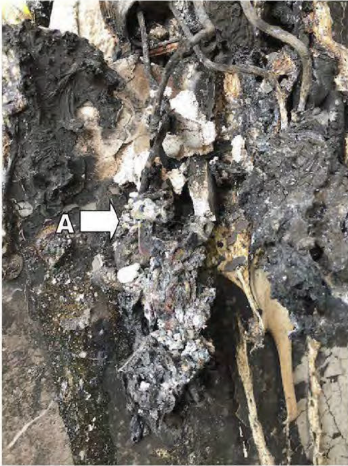
Closer view of Solar Array DC Isolator showing: A – Remains of DC cables with Isolator terminal attached
