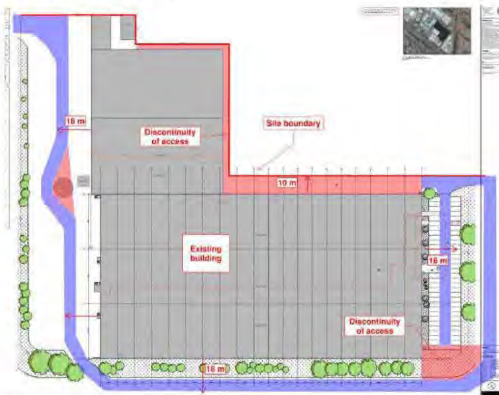
FIGURE 13: VEHICULAR PERIMETER ACCESS
