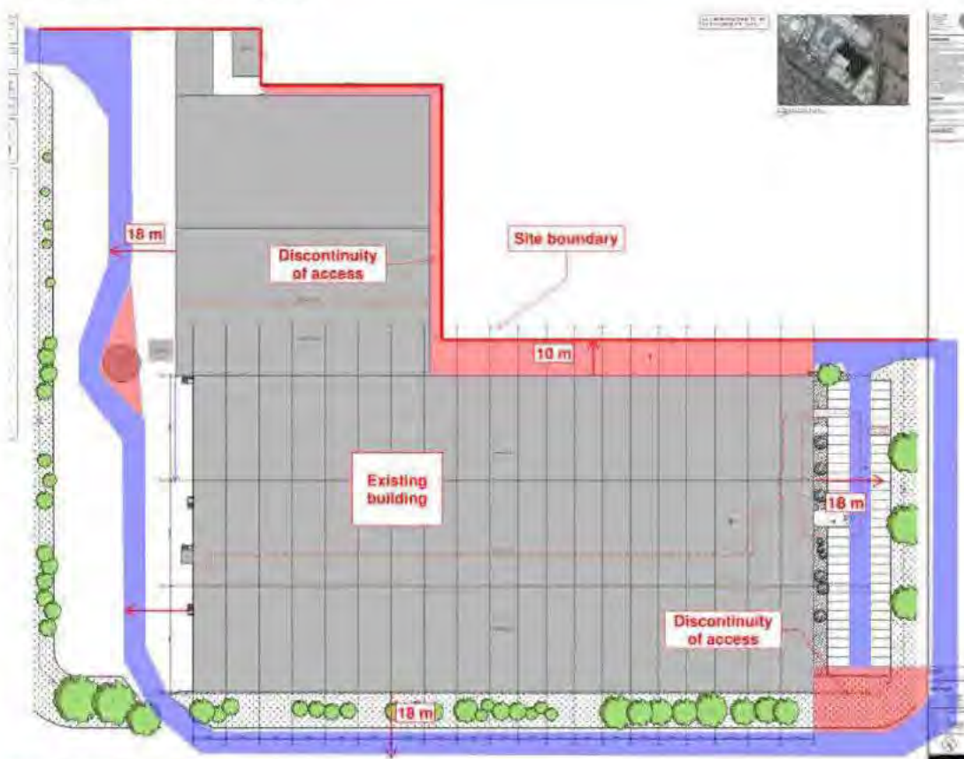
FIGURE 4: VEHICULAR PERIMETER ACCESS
