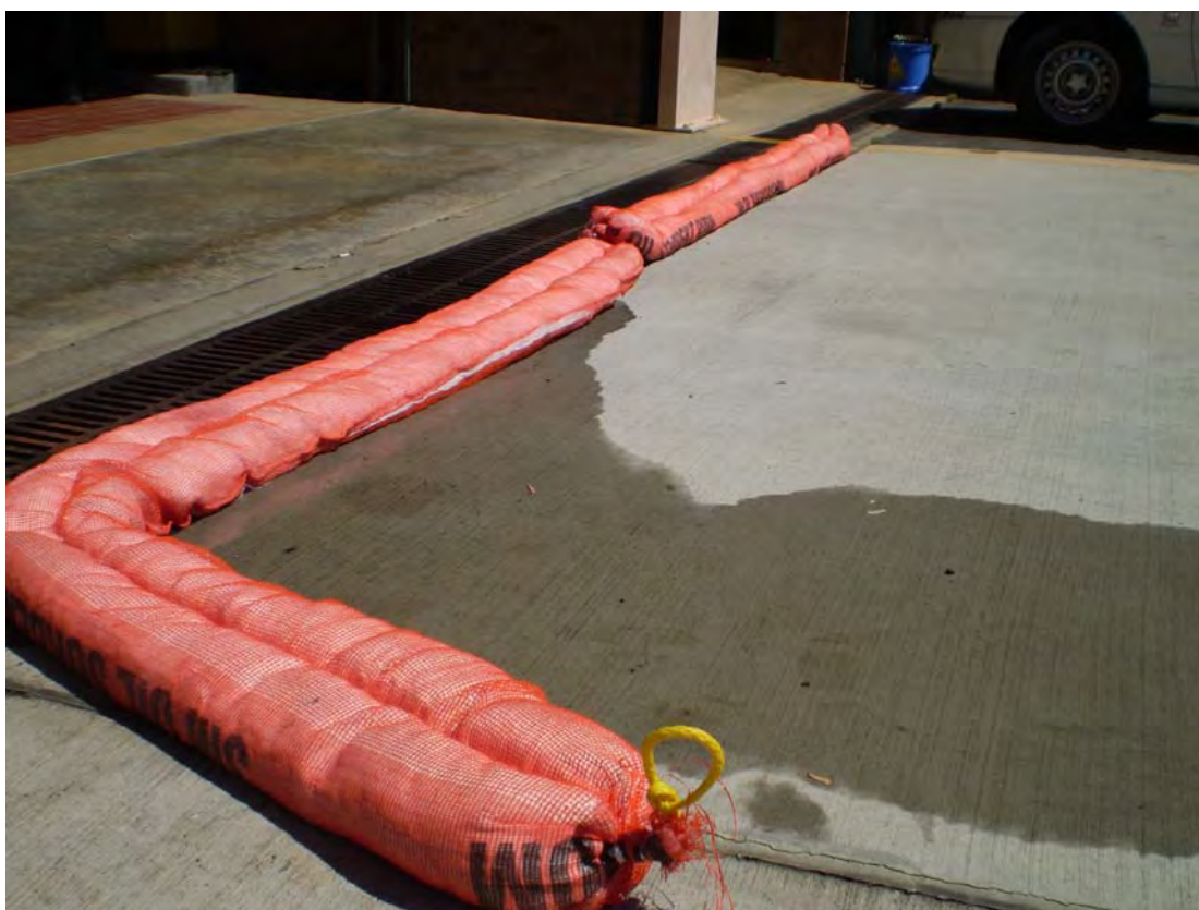
Diverting a spill away from storm water drains
