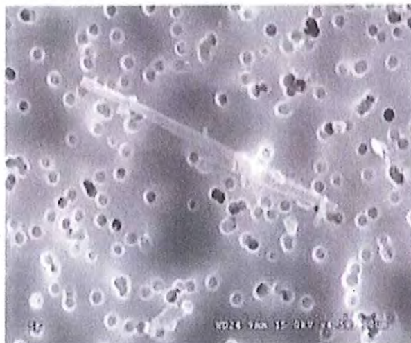
Fig 3: SEM micrograph of a typical Amosite fibre, using the backscattered electron signal (BSE)
