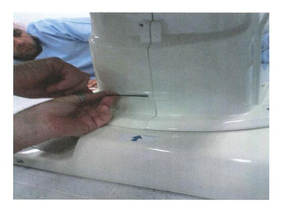
All the cover screws & self tappers should only be finger tightened before final locking down.
