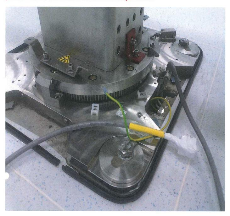
9; Connect the control wire, quick coupler, connect the earth wire to the base of the bed.
