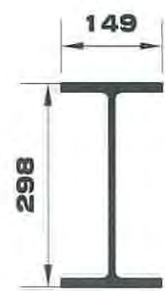
BEAM B2 310 UB 32 SCALE 1:10
