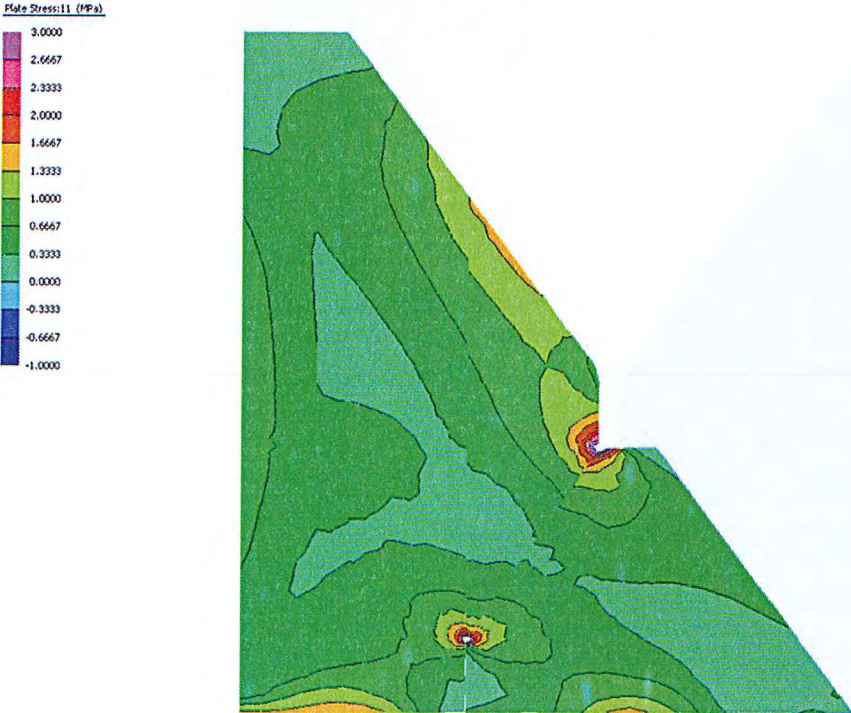
Figure 4.69 SMADRE-4734 – West & Vertical Components – Maximum Stress Envelope – Maximum Principal Stress
