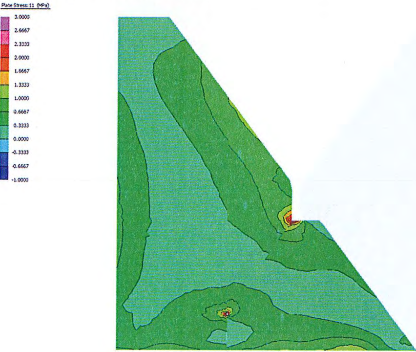
Figure 4.61 NORTH-WON – West & Vertical Components – Maximum Stress Envelope – Maximum Principal Stress
