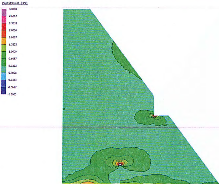
Figure 4.61 NORTH-WON – West & Vertical Components – Maximum Stress Envelope – Maximum Principal Stress
