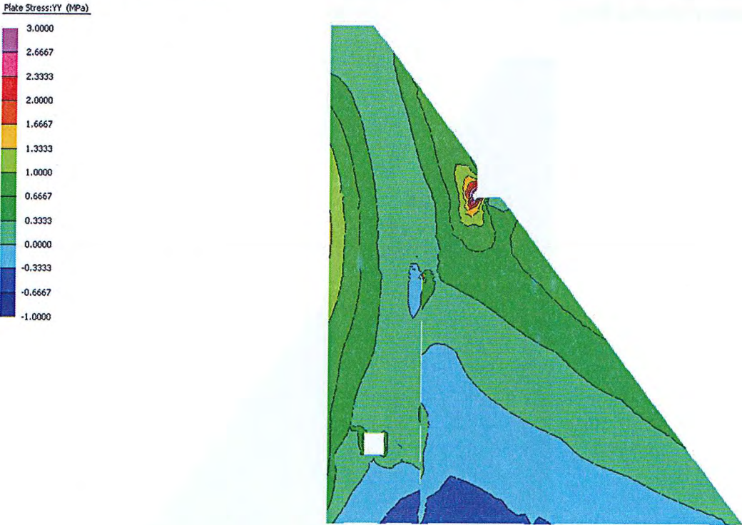
Figure 4.29 NORTH-WON – South & Vertical Components – Maximum Stress Envelope – Vertical Stress
