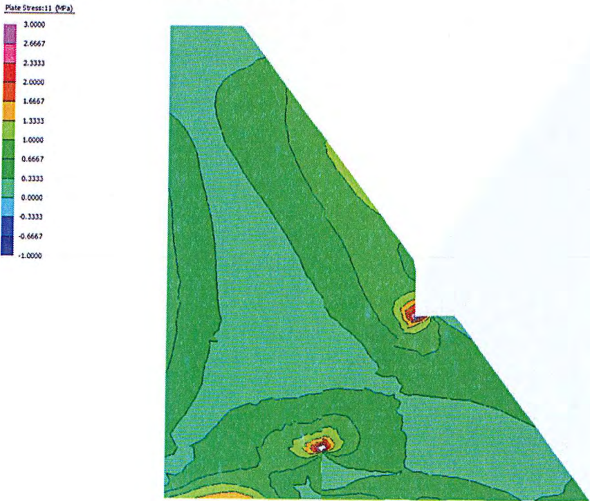
Figure 4.57 NORTH-WON – South & Vertical Components – Maximum Stress Envelope – Maximum Principal Stress
