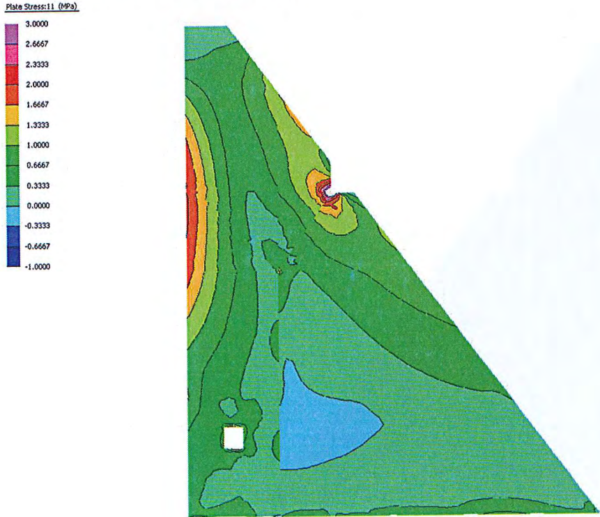
Figure 4.39 SMADRE-4734 – West & Vertical Components – Maximum Stress Envelope – Maximum Principal Stress
