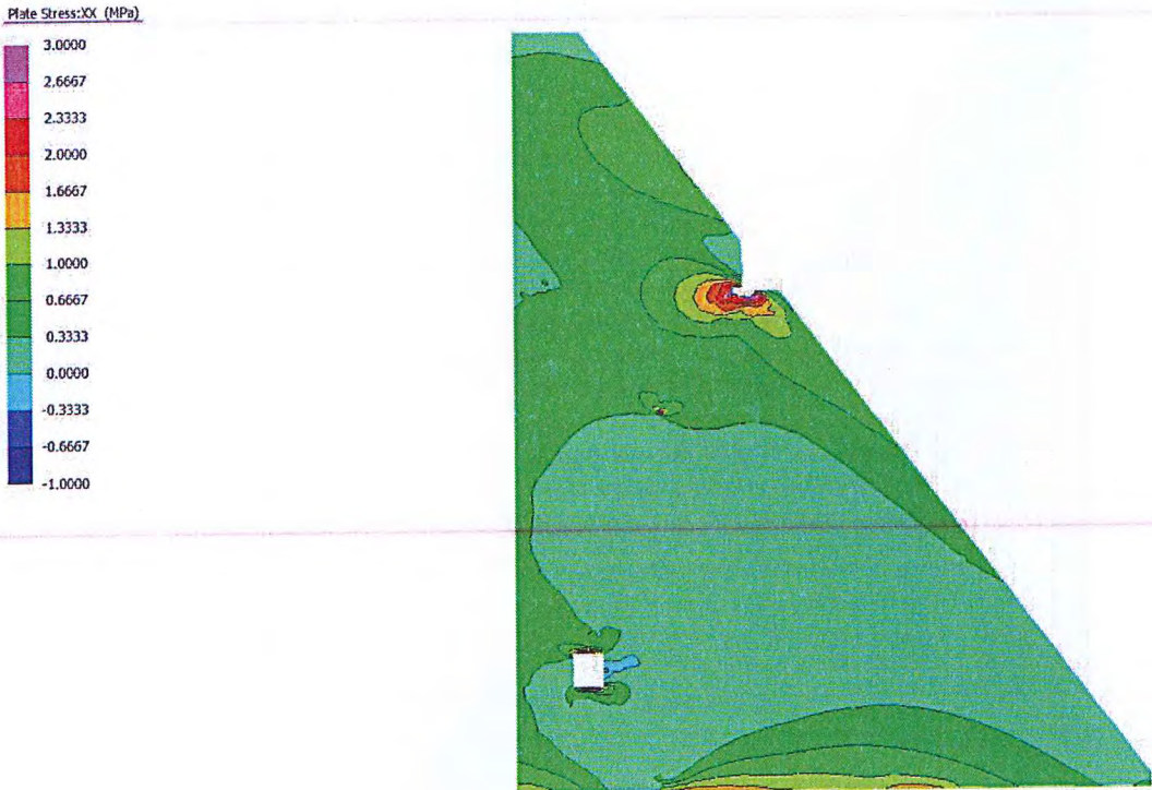
Figure 4.39 SMADRE-4734 – West & Vertical Components – Maximum Stress Envelope – Maximum Principal Stress
