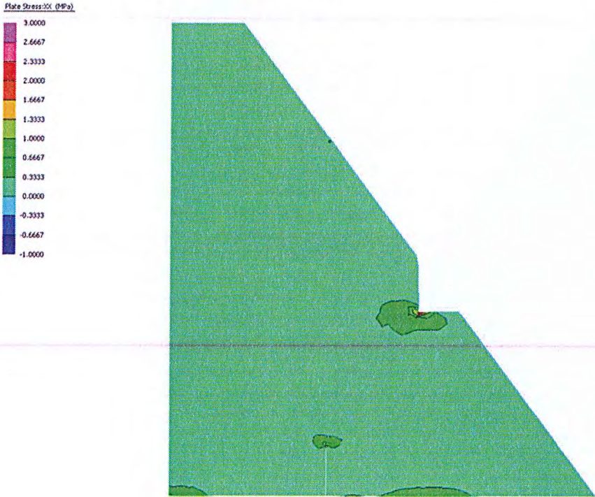
Figure 4.69 SMADRE-4734 – West & Vertical Components – Maximum Stress Envelope – Maximum Principal Stress
