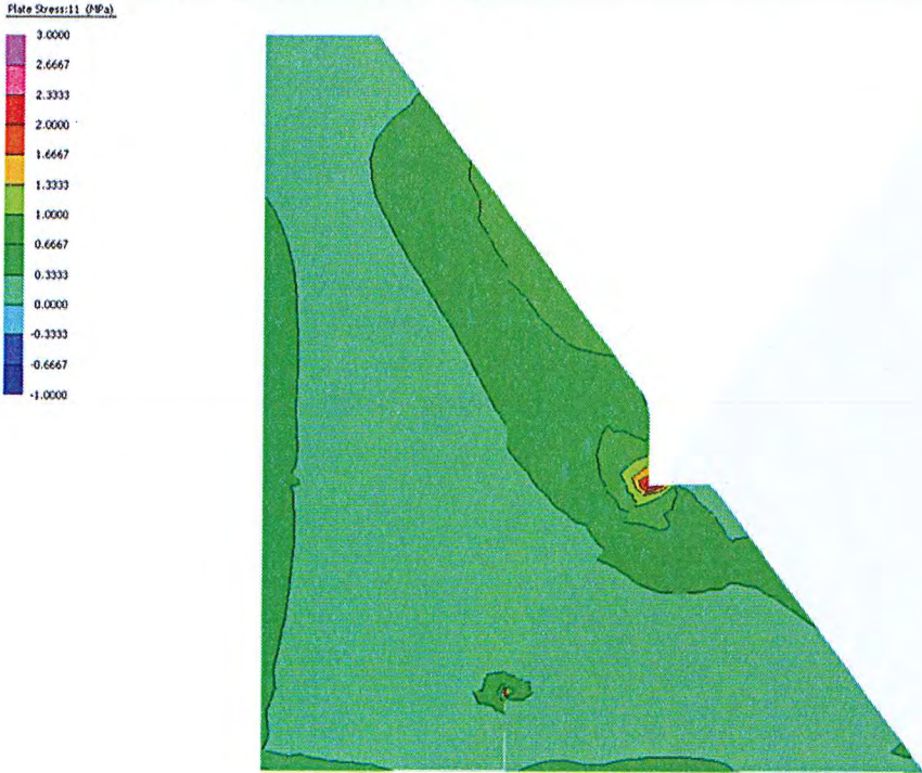
Figure 4.65 SMADRE-4734 – North & Vertical Components – Maximum Stress Envelope – Maximum Principal Stress
