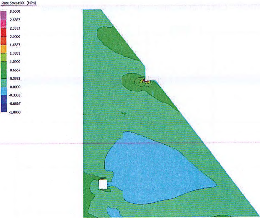
Figure 4.42 SMADRE-4734 – West & Vertical Components – Maximum Stress Envelope – Upstream Downstream Stress
