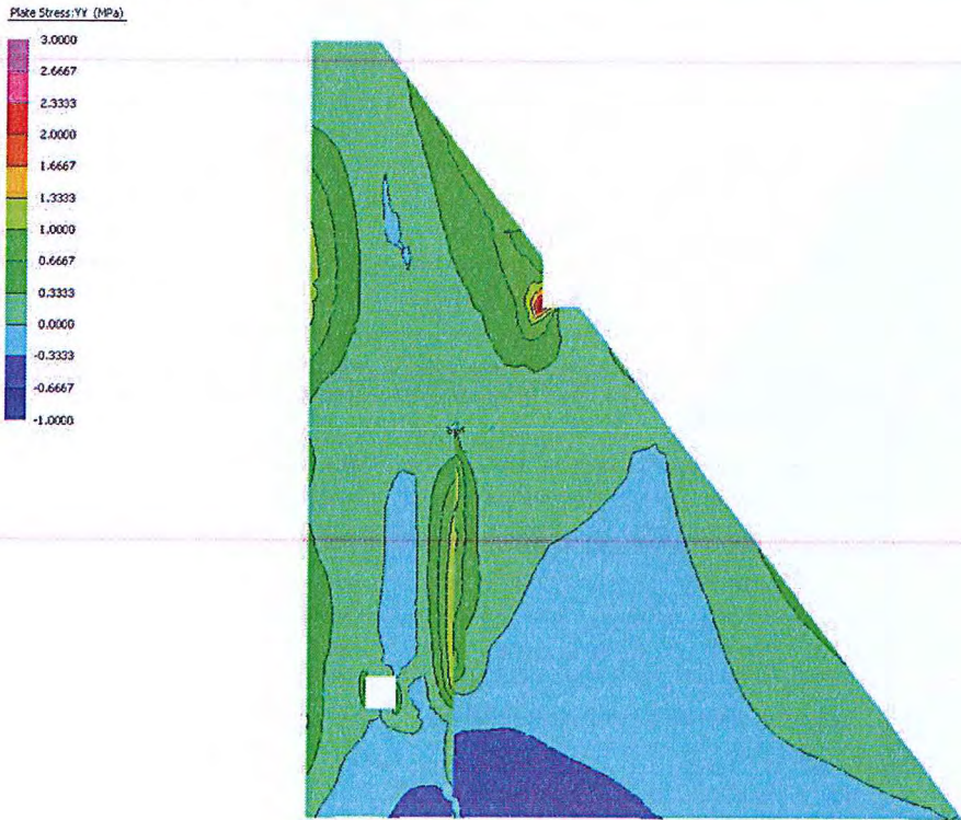
Figure 4.93 NORTH529 – North & Vertical Components – Maximum Opening of Horizontal Crack at U/S Face (6.79s) – Maximum Principal Stress
