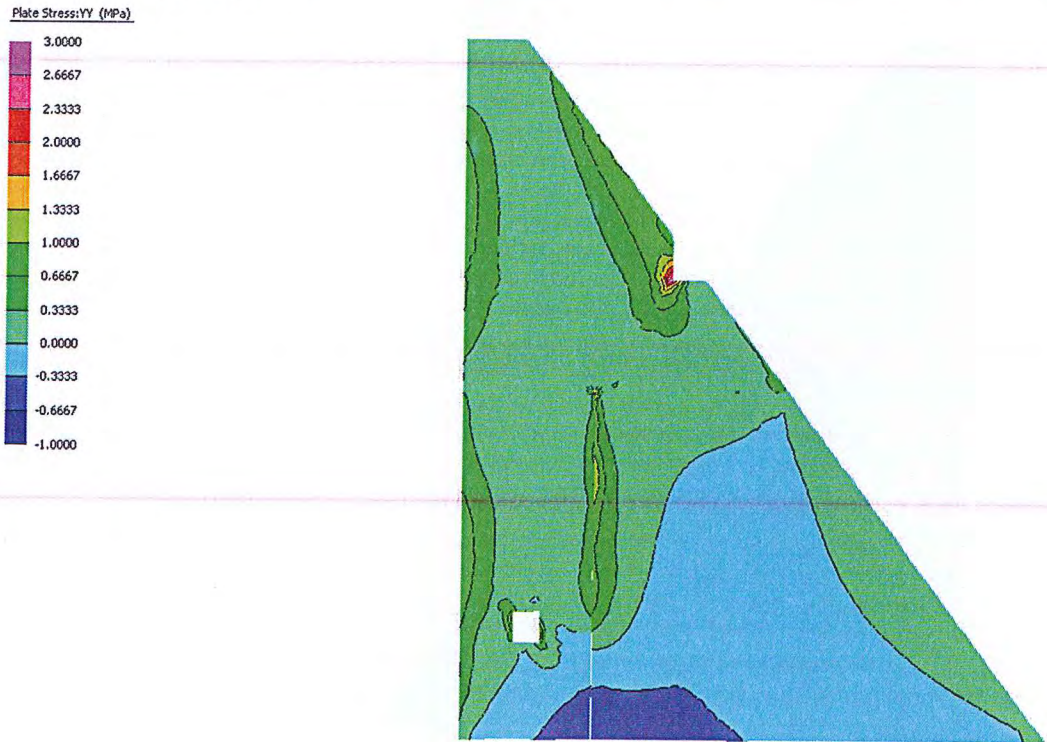
Figure 4.97 NORTH-WON – South & Vertical Components – Maximum Opening of Horizontal Crack at U/S Face (8.805s) – Maximum Principal Stress
