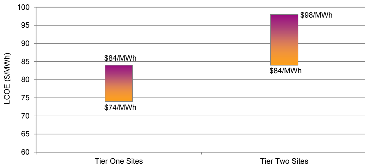
Figure 5 - Estimated LCOE ranges for Tier One and Tier Two wind energy sites
