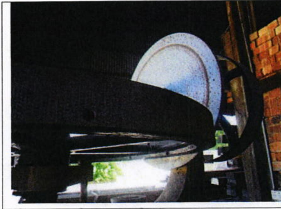
Photograph 9: B - Large brake pad to top of old brick making machine Refer Sample: 3617 - 103 - A1
