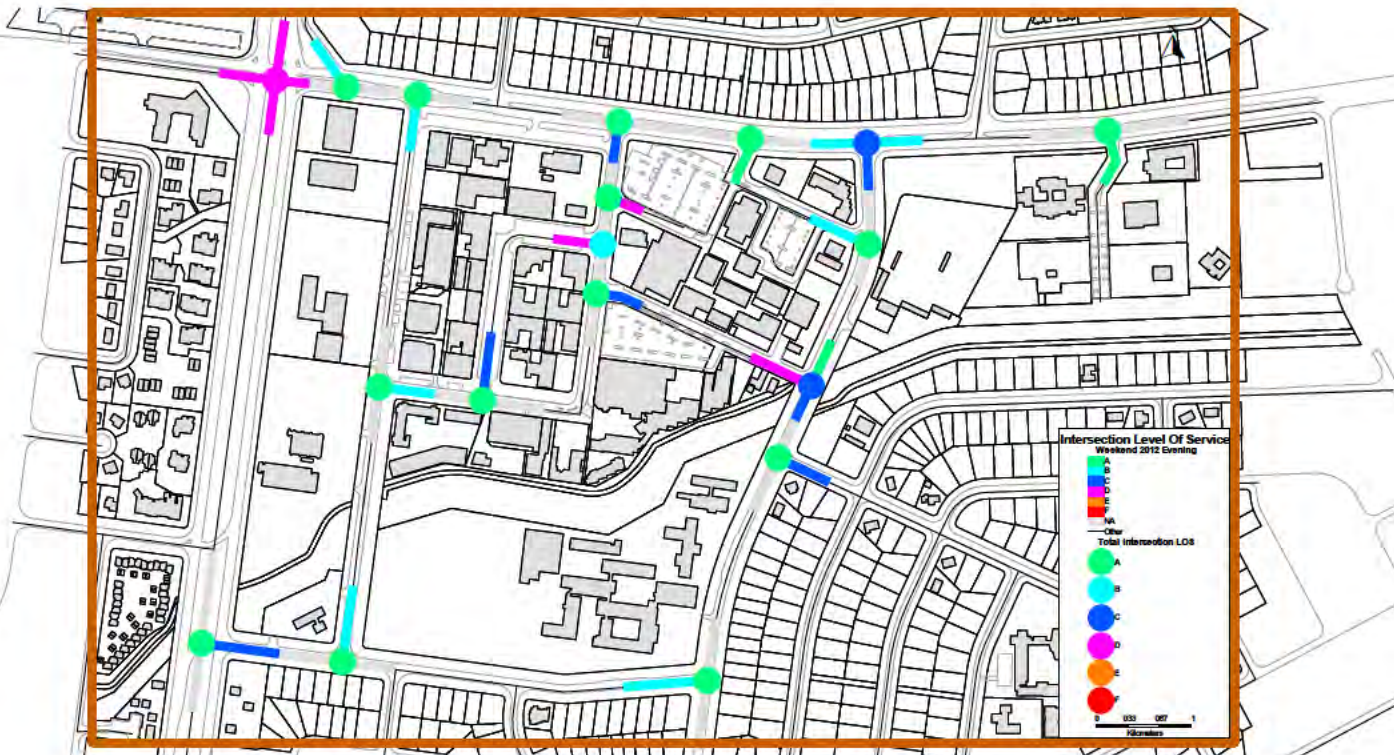
Figure 24: Intersection Level of Service – 2012 Weekend Evening Peak
