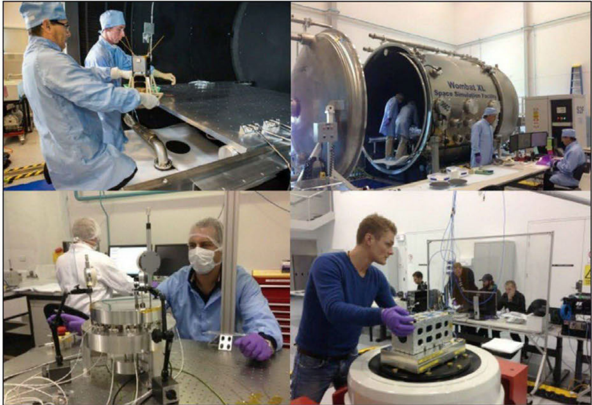
Figure 1: The AITC National Space Test Facility consists of state of the art equipment and laboratory facilities specifically for the advancement of space industry and research applications. [Top left] QB50 satellite testing in the Wombat XL; [Top right] The large TVAC or WOMBAT XL is Australia's largest space environment chamber; [Bottom right] Vibration testing of the UNSW Canberra Space Buccaneer satellite and; [Bottom left] Metrology testing of a deformable mirror.
